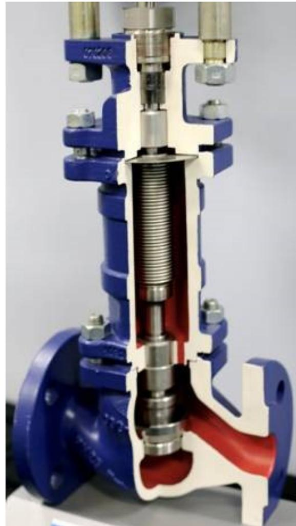
statically formed into a bellow with rounded and widely spaced folds. The welded leaf-type bellow is made by welding washer-like plates of thin metal together at both the inner and outer circumference of the washers, like plates. A welded leaf bellow has more folds per unit length as compared to formed bellows. Thus, for the same stroke length, formed bellows are two to three times longer than their welded-leaf counterparts.
