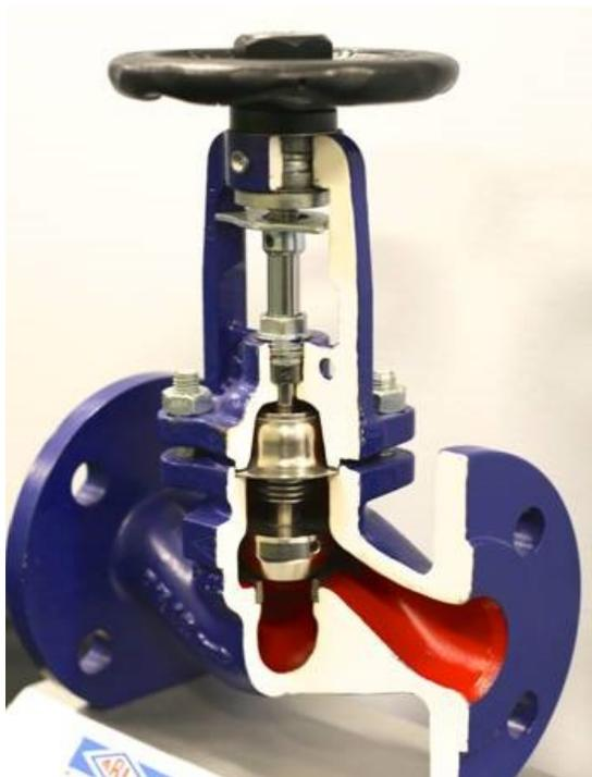
been put into hot oil applications. The bonnet and hand wheel are designed to dissipate heat, as is the bell design of the bellows. This entraps air, which is a very good insulator—think of a wool sweater or down parka. Each of these has many little air pockets that create the insulation.
